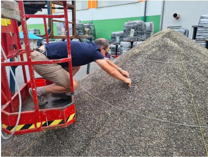
Photo 10 – Sampling from middle layer (static sampling)
