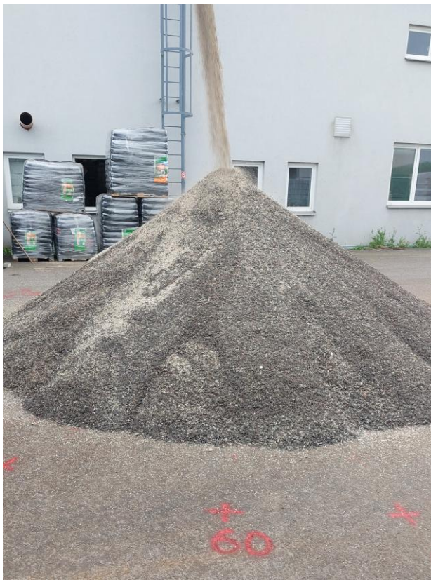
Photo 6 – Constituion of a cone (blend 1)
