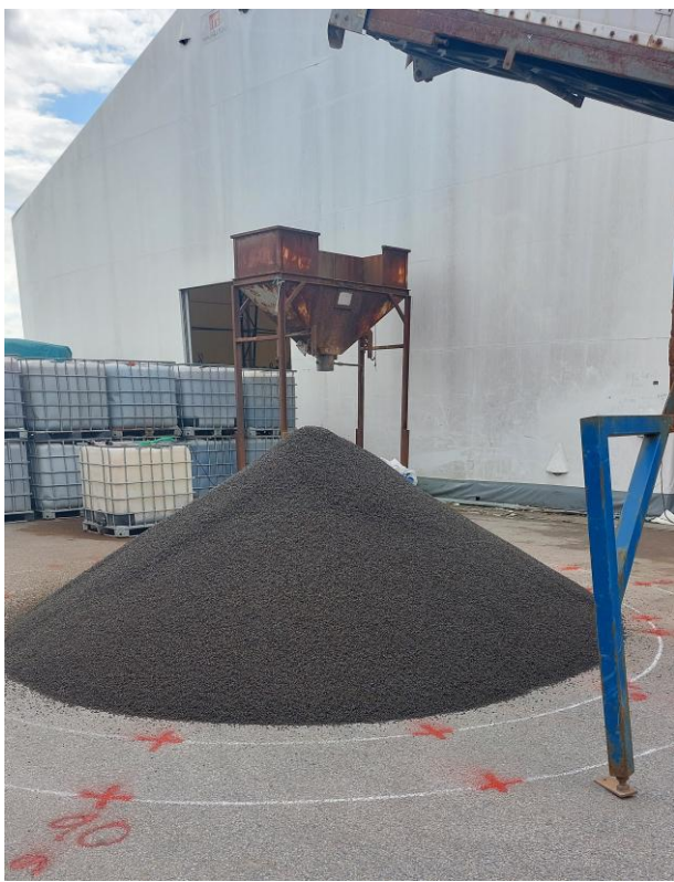
Photo 5 – Constituion of a cone (dried pelleted manure)
