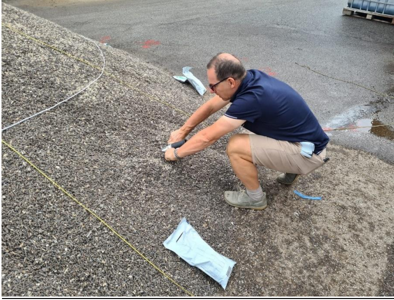
Photo 11 – Sampling from lower layer (static sampling)
