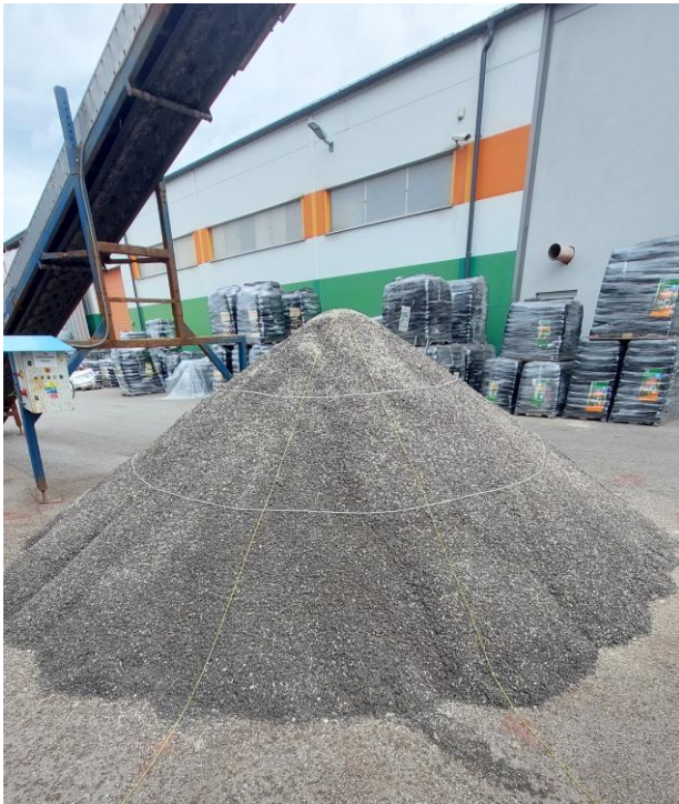
Photo 8 – Determination of sampling units (static sampling)
