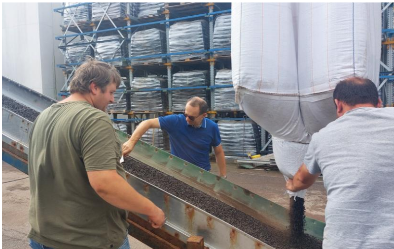
Photo 4 – Dynamic sampling from a conveyor belt
