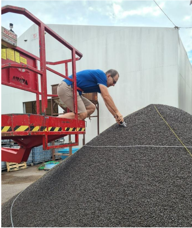
Photo 9 – Sampling from upper layer (static sampling)
