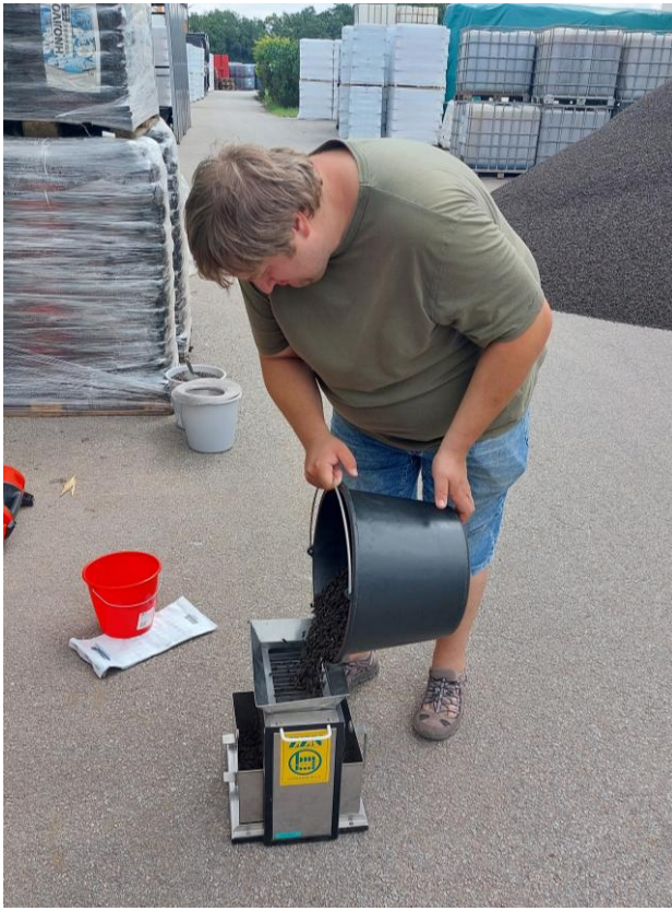
Photo 7 – Reduction & preparation of final samples (dynamic sampling)
